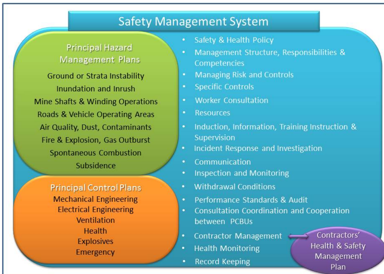
Figure 2: The safety management system
