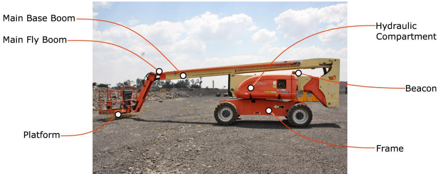
Figure 2 – Boom-Type Elevating Work Platform – Right profile
