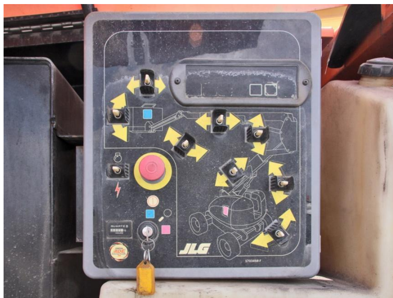
Figure 5 – Boom-Type Elevating Work Platform – Ground control panel example
