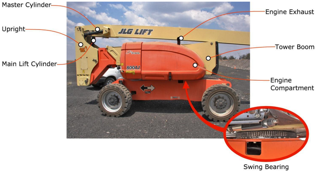
Figure 4 – Boom-Type Elevating Work Platform – Left profile
