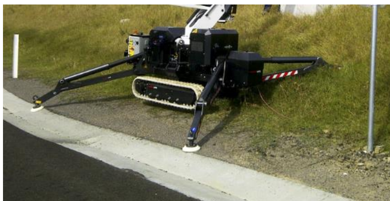
Figure 18 – Outriggers on slope
