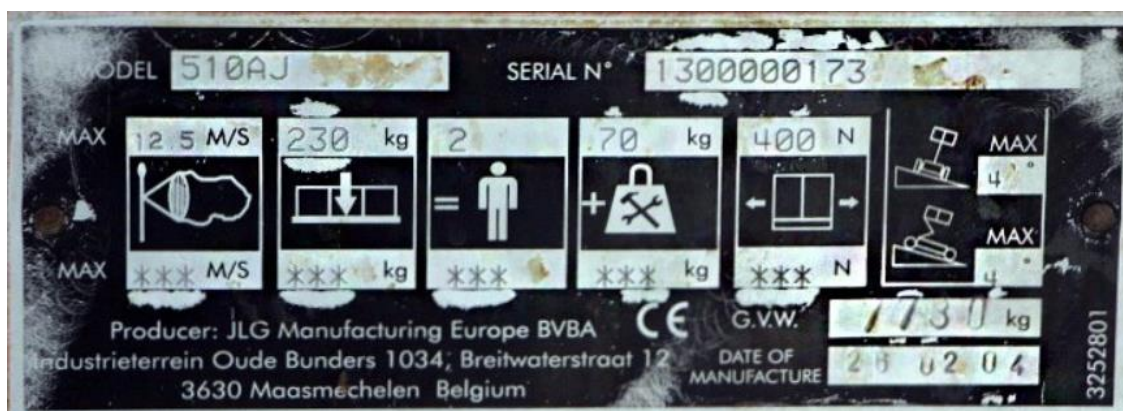
Figure 7 – EWP Data Plate Example
