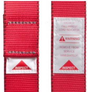
Figure 44 – Inspection tag visible from fall
