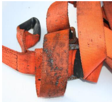
Figure 43 – Damage from contaminates
