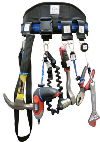
Figure 78 – Tool belt with lanyards on tools
