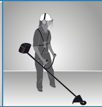
The heaviest part of this brush cutter is located behind the wrists and the weight is supported by a harness.
