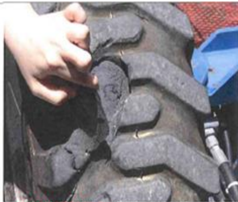
UNACCEPTABLE - Severe tread damage – complete lug can be peeled away
