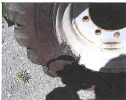
UNACCEPTABLE - Bead damage.
