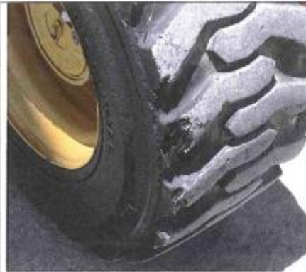
Non-critical - Small amount of tread missing
