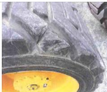
Non-critical - Small amount of tread missing but outer case is not damaged.
