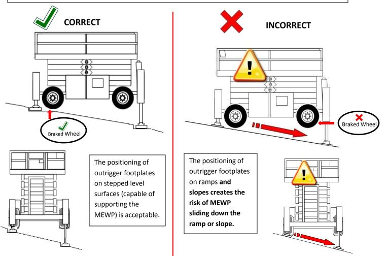
A competent person shall assess slope and surface conditions before setting up machine on a slope.
