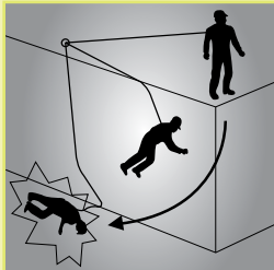
Figure 37: During 'swing down' the length of the lanyard and positioning of the anchor allow contact with the ground.
