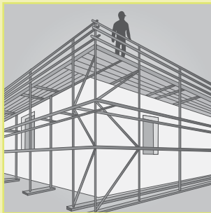
Figure 7: Perimeter scaffold with a fully decked working platform, guardrails and toeboards.
