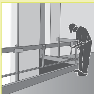
Figure 14: This temporary guardrail is being used instead of mesh to permit work on curtain wall securing bolts.
